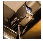
Overload prevention device prevents lifting excessive loads
