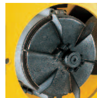
Spring pressure disc brake.
